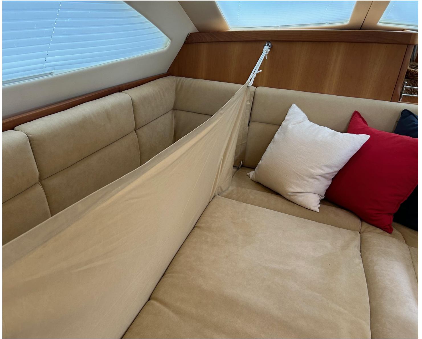
Lowering the saloon table allows for an inset mattress and secure sea-berth
